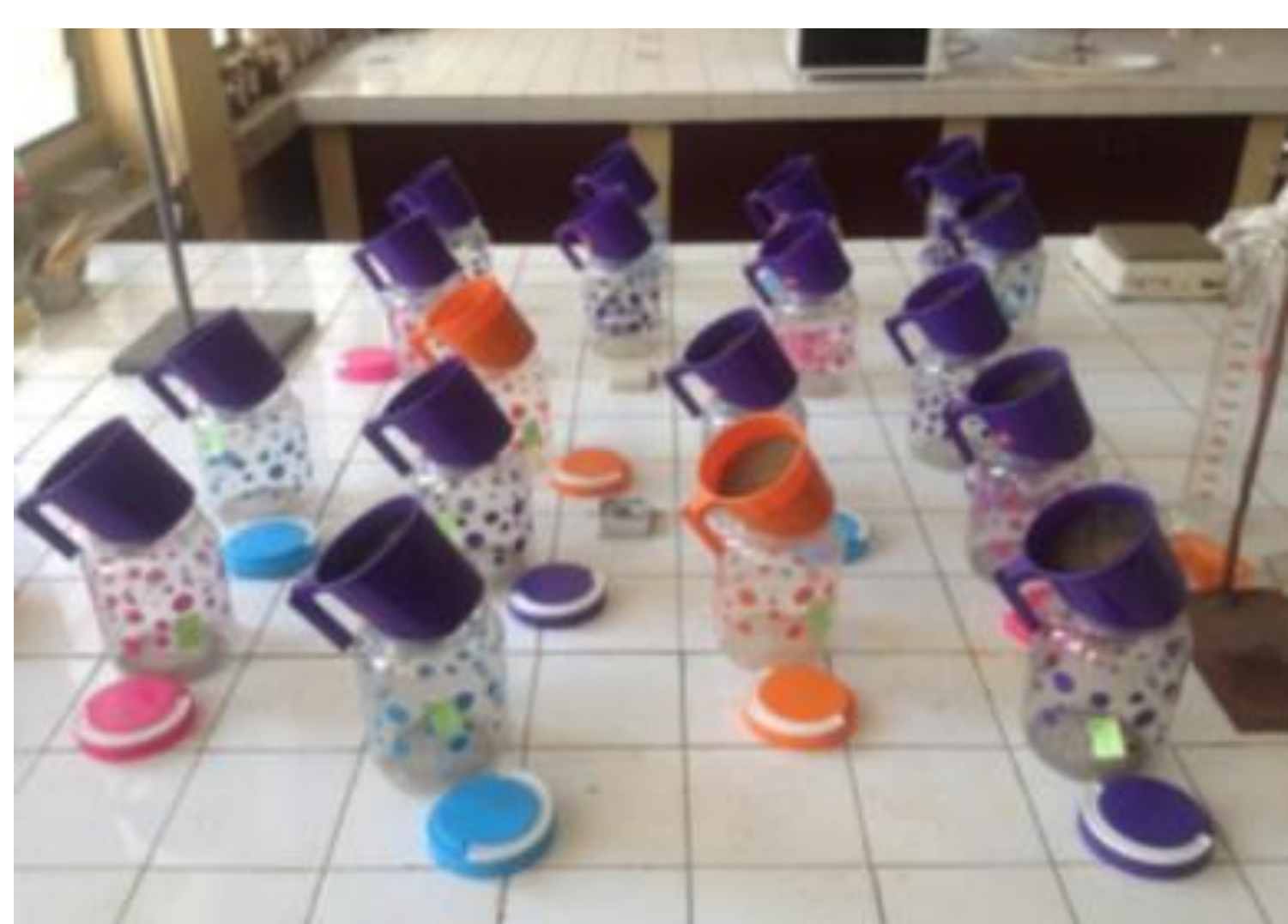
Fig. 3. arrangement of 18 permeable cups (dimension = 700 ml) associated with 16 jars to collect the percolating.
